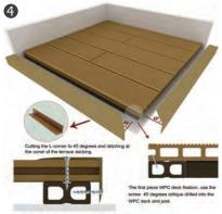
Fixed the L corner with screws to complete the install
